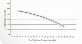
Following installation, MODIO was custom adjusted for the Lido's guest rooms using Maestro software. This application ensures the sound follows an optimal masking curve, regardless of a room's interior layout, finishings and furnishings—environmental factors that would otherwise introduce variations that reduce masking performance and occupant comfort.
